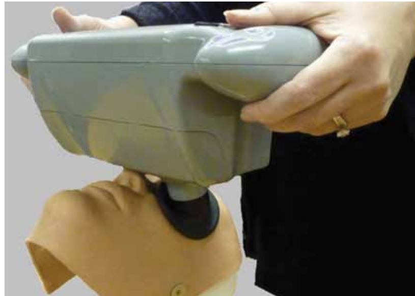
The prototype instrument being used in the study will aid eye banks in identifying previous refractive surgery that could have an impact on the transplant suitability of a donor cornea.
